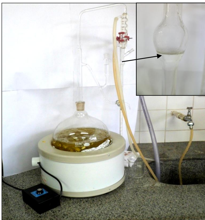
Figura 13: Extrator de Clevenger
