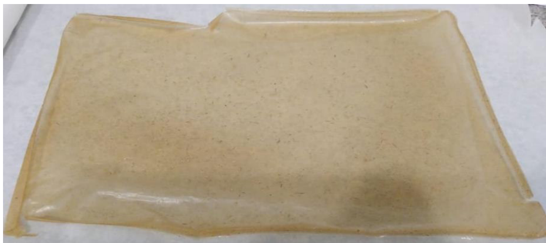
Figure 1. Photograph of a composite alginate film with added starch and babassu coconut fibers (formulation 13).
